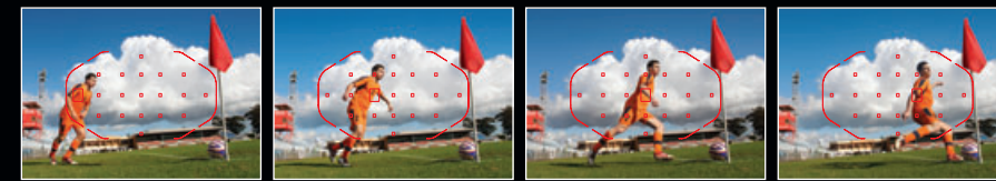
AF point display sample for 19-point automatic selection AF and AI Servo AF (EOS 7D)
