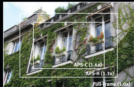
When using the same lens with different cameras, the angle-of-view varies depending on the sensor size.
