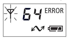
The LCD panel will show <ERROR> and the error number. The < ♥> and <POWER> lamps will also blink.
