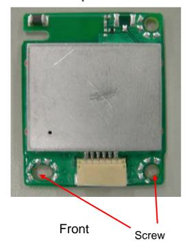
When you install the module into your final set, please leave space between the module and the metal plate more than 4mm. (Except the screw-hole areas.)
