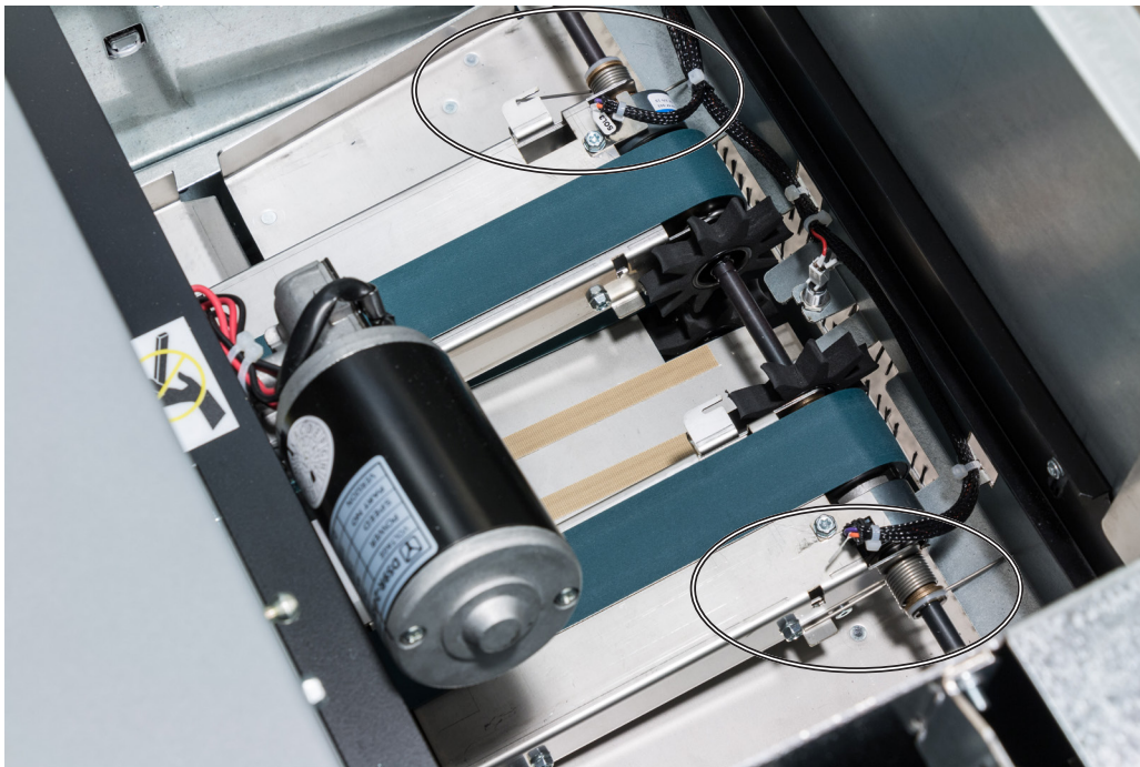
operator side spring in lower position
