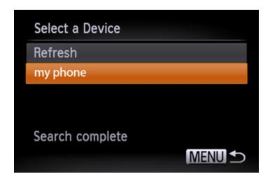
12. Press the <▲><▼> buttons to choose the Android smartphone's nickname, and then press the <₩>> button.
