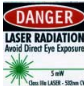
Figure 3-2. CA-320A Laser warning label.
