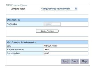
**Configure Option:** Provide two ways: PBC (Push-Button Configuration) and PIN code.
