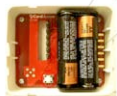
The button is located on the radio/logic board found inside the Cover Assembly.
