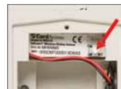
The button is located inside the battery compartment.
