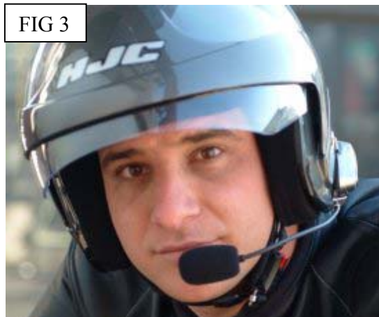
microphone should be placed just slightly off the corner of your mouth
