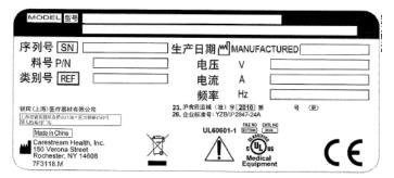
This label shows the serial number and model number of the laser imager along with other important data items. (The label shown above is an example serial plate label.)
