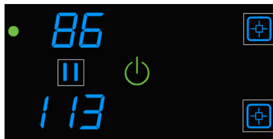
Figure 1: Display screen: normal state, processing a print job from the upper supply. In this example, there are 86 sheets of film in the upper cartridge and 113 sheets in the lower cartridge.
