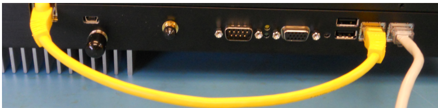
Figure 17: Carlson Basestation Ethernet Cable Connections
