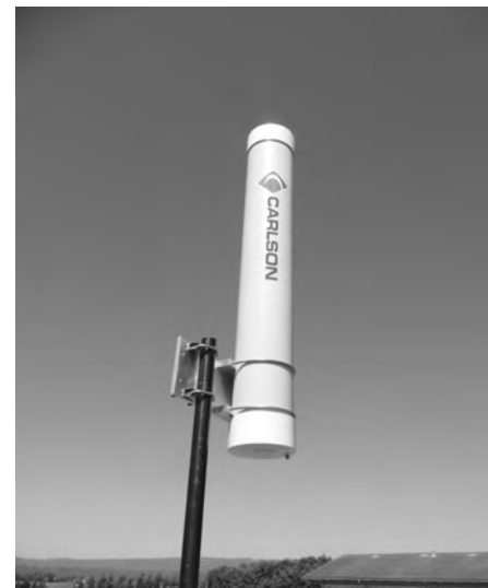
Figure 21: Basestation Omni Antenna
