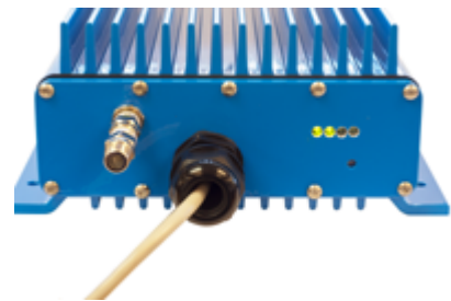
Figure 21: RuralConnect® CPE Bottom
