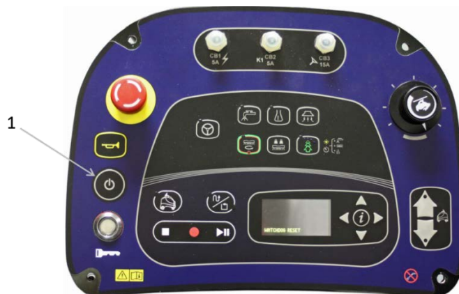
Figure 4B1. ON/OFF Switch on Control Panel
