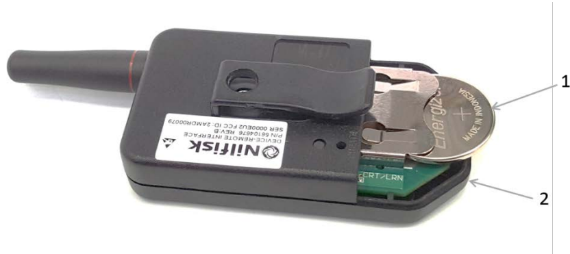
Figure 4G7. RID Final Battery Removal
