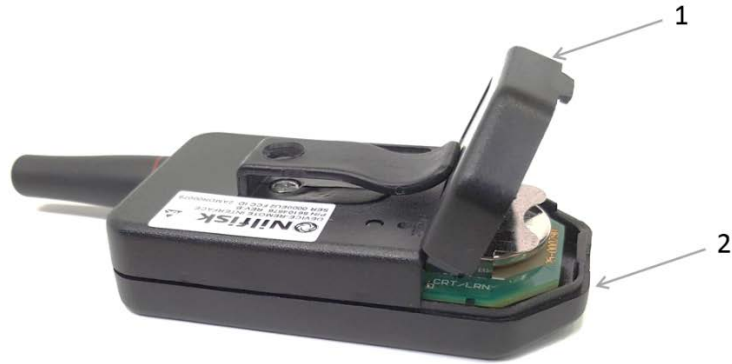
Figure 4G10. Replacing Battery Cover
