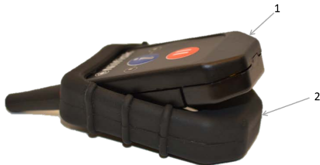
Figure 4G12. Inserting RID Into Cover
