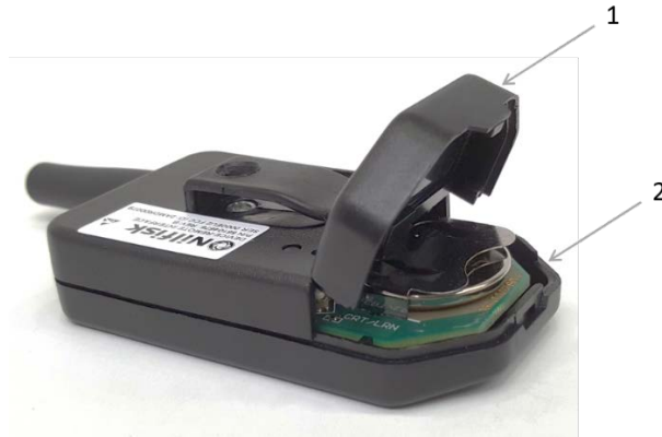
Figure 4G4. RID Battery Cover Raised From Body
