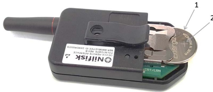
Figure 4G8. Checking RID Battery Polarity
