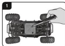
Using a screwdriver, remove the cover of the battery compartment in the Carrera RC car.
