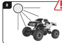
Do not expose the Carrera RC vehicle to direct sunlight. To avoid the electronics in the car overheating, when temperatures are above 35 °C, regular short pauses in operation are essential.
