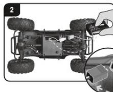
Connect the end of the cable from the Carrera RC vehicle with the charged battery. Put the battery in place.
