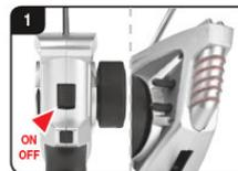
When the controller is switched on, the red LED lamps at the front of the controller are lit. When the control LED flashes, the 9-volt battery in the controller must be replaced.
