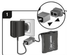
First connect the Carrera RC rechargeable battery to the battery charger supplied. The connection terminals between the battery and the charger are designed to prevent connection with the wrong polarity. Connect the charger to a power source.
