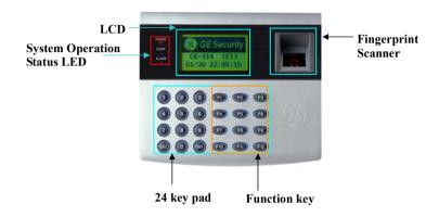
Figure: Description of GE314 Front Panel
