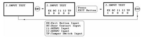
The 5digit shows the input status and "0" indicates that the input port is open circuit and "1" indicates that the input port is short circuit to ground level.
