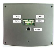
Figure: Connector Layout
