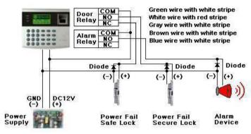
Figure: Door Lock, Alarm Device Connection
