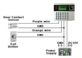
Figure: Input Device Connection
