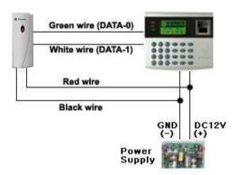
Figure: External Reader Connection
