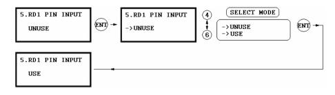
This function is for USE/UNUSE the keypad inputs for the Reader#1. The default setting is UNUSE the keypad inputs. If you want to access the door by entering the user ID by keypad, set this mode USE. You have to set this mode USE when the unit is operating with Password.
