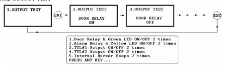
. The first two tests are for the output relays (Door Relay and Alarm Relay) test. You can hear the mechanical sound of relays and LED will blink. Following two tests are for TTL#1 and TTL#2 output testing. The last test is for the Internal Buzzer test and you can hear two beep sounds.
