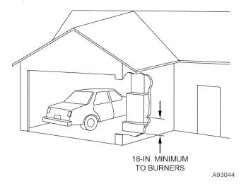
Fig. 16—Installation in a Garage
