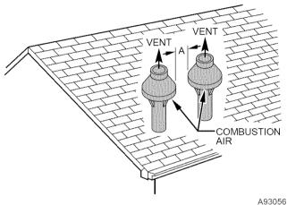
Fig. 44—Concentric Vent and Combustion-Air Roof Termination (Dimension "A" is Touching or 2-in. **Maximum Separation**)
