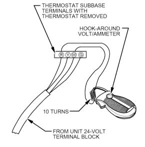
EXAMPLE:  $\frac{5.0 \text{ AMPS ON AMMETER}}{10 \text{ TURNS AROUND JAWS}} = 0.5 \text{ AMPS FOR THERMOSTAT SETTING}$
