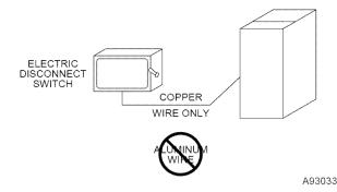
Fig. 29—Disconnect Switch and Furnace
