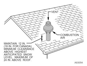
Fig. 38—Concentric Vent and Combustion-Air Roof Termination (Preferred)
