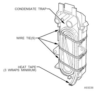
Fig. 49—Condensate Trap Heat Tape
