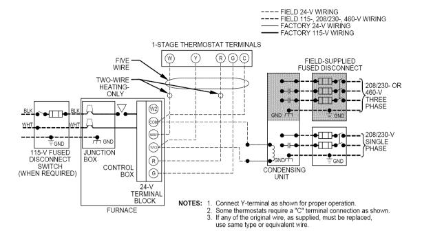
Fig. 27—Typical Heating and Cooling Application Wiring Diagram 1-Stage Thermostat and Condensing Unit
