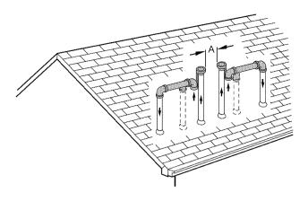
Fig. 43—Rooftop Termination (Dimension "A" is Touching or 2-in. Maximum Separation)
