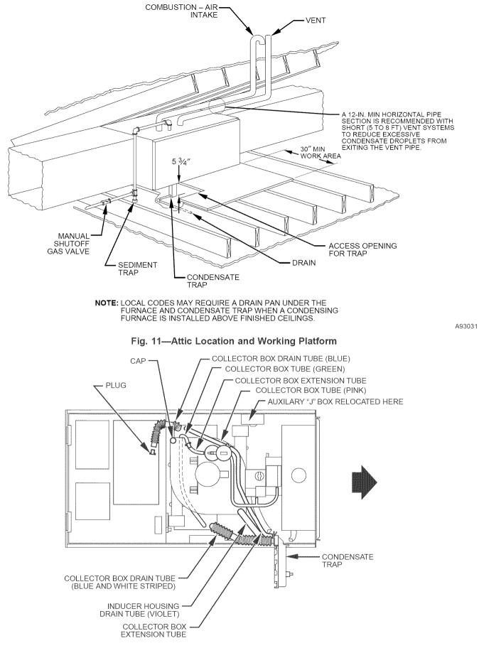
Fig. 12—Horizontal Right Tube Configuration
