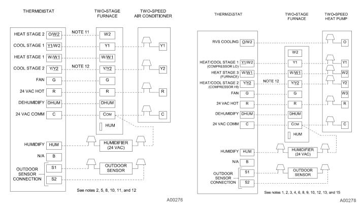
Fig. 52B—Two-Stage Furnace with Two-Speed Air Fig. 52D—Two-Stage Furnace with Two-Speed Heat Conditioner Pump (Dual Fuel)
