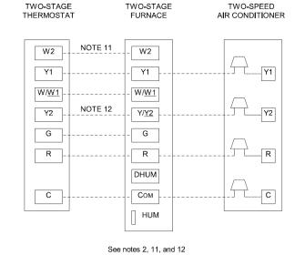
A00281 Fig. 52G—Two-Stage Thermostat With Two-Stage Furnace and Two-Speed Air Conditioner
