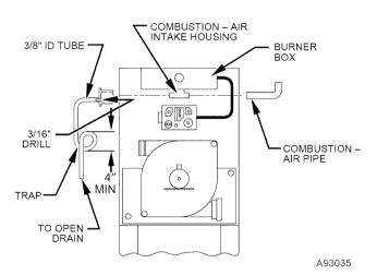
Fig. 36—Air Intake Housing Plug Fitting Drain
