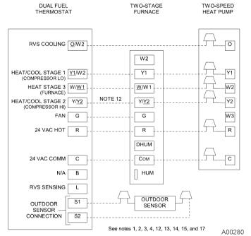
Fig. 52F—Dual Fuel Thermostat With Two-Stage Furnace and Two-Speed Heat Pump
