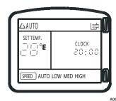
The fan speed can be selected by pressing the **FAN SPEED** button. **NOTE:** When the unit is on, the fan will run continuously in cooling or heating. When in heating, there might be situations where the fan will slow down or shut off to prevent cold blow.
