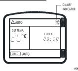
When the air conditioner is not in operation, the remote control will display the last set point, mode and time.
