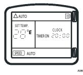
This function will allow the unit to start automatically at the set time. The TIMER ON can be set while the unit is on or off.
