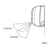
The horizontal louvers can be adjusted using the remote control and can be set to be stationary or moving continuously.
