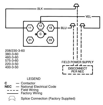
Fig. 5 — Power Wiring Connections
