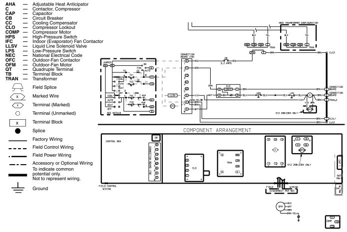
Fig. 6 — Typical Control Wiring Connections/Component Arrangement (38AK Shown)
