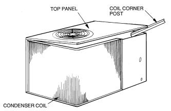
Fig. 11 — Propping Up Top Panel
