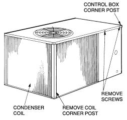
Fig. 10 — Cleaning Condenser Coil
