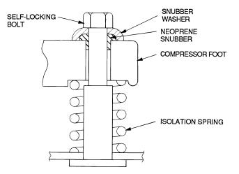
Fig. 4 — Typical Compressor Mounting (38AKS Units)
