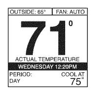
ING on page 26.) The programmed cooling temperature will appear in the lower right screen with the text, "COOL AT."
