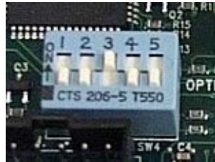
Figure 2: SW 4 switch (Switch 3 is shown in the ON position).
