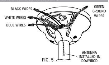
**Step 13.** Tuck all the wiring back into the canopy, leaving space for the canopy hatch screw to pass through without interfering with the wires.
