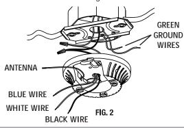
Step 7. Push the wire nuts through the center opening in the Crossbar Mounting Bracket, so they will not interfere with the canopy and receiver installation. Route the house ground wire and the Crossbar Mounting Bracket ground wire through the hole in the center of the receiver. (FIG. 3)
