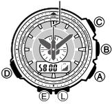
In the Altimeter Mode, the part of the watch's dial from 11 o'clock to 7 o'clock acts as an altitude differential scale. The second hand points to a place on the scale that indicates the difference between the altitude at a start point set by you and the altitude at your current location. The altitude differential indication is updated each time the watch takes an altitude reading.
