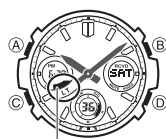
Auto light switch on indicator
