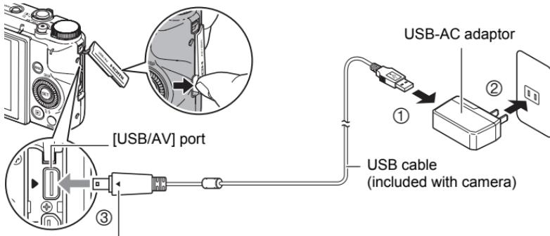
Making sure that the ▶ mark on the camera is aligned with the ◀ mark of the USB connector, connect the cable to the camera.
