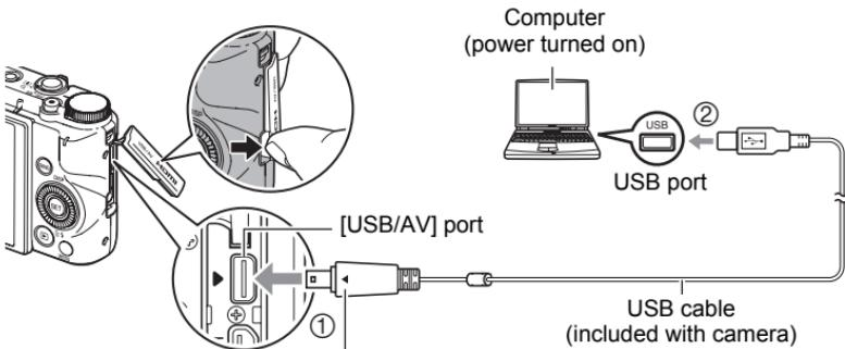
Making sure that the ▶ mark on the camera is aligned with the ◀ mark of the USB cable connector, connect the cable to the camera.
