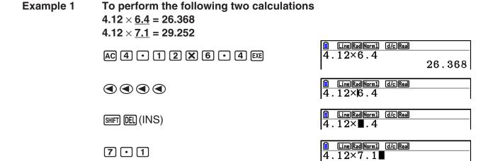
After you press (AC), you can press (AC) or (To recall previous calculations, in sequence from the newest to the oldest (Multi-Replay Function). Once you recall a calculation, you can use (AC) and (AC) to move the cursor around the calculation and make changes in it to create a new calculation.
