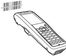
2. The laser emits light and scans the bar code. If scanning is completed normally, Indicator 2 displays a green light.
