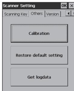
4. Tap the [Calibration] button. The display appears as shown at right.
