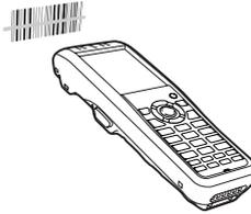
2. The Handheld Terminal reads the code by emitting laser and red lights. Indicator 2 (read operation indicator lamp) lights in green when the reading is successful.
