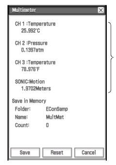
Shows sampled values in realtime for the channels specified on the [Multiple] tab. Nothing is shown for unused channels.
