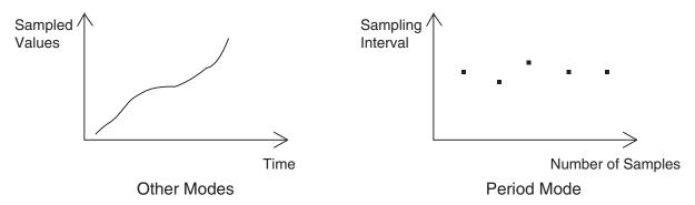
Unlike the other modes that record time and sampled values, the Period Mode records the number of samples (1st sample, 2nd sample, and so on) and the intervals between samples. For details, see "Period Mode Parameters" on page 3-7.
