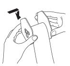
**6** Place the take-up reel into place behind the printer, above the roll paper.
