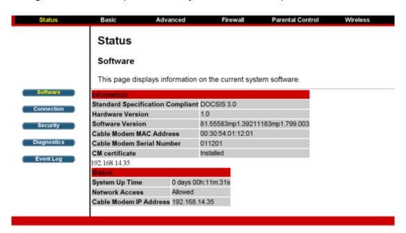
If Network Access shows "Allowed," then your cable service provider has configured the CBV3843Z4S to have Internet connectivity. If Network Access shows otherwise, you may not have Internet access, and please contact your cable service provider for assistance.
