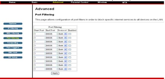
To enable port filtering, enter the **Start port** and **End port** for each range. Then select its protocol form the drop-down list and check the **Enable** box, and click **Apply** button. To block only one port, set both Start and End ports the same.
