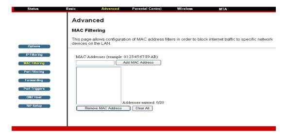
To enable MAC filtering feature of CBV3843Z4S, enter the MAC address of the LAN device and click **Apply** button.
