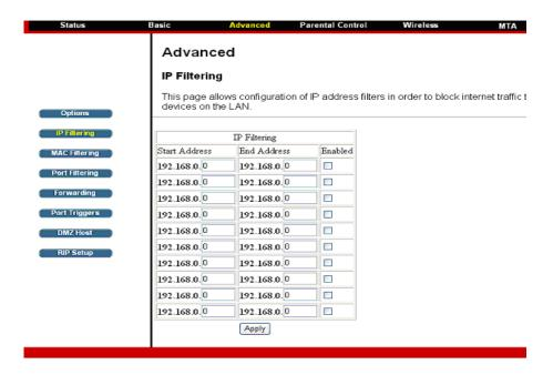
To enable IP Filtering feature of CBV3843Z4S, check the **Enable** box and click **Apply** button.
