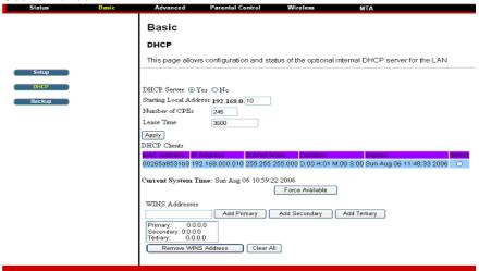
With this function activated, your cable service provider's DHCP server provides one IP address for the CBV3843Z4S, and the CBV3843Z4S is DHCP server provides IP addresses, starting at the address you set in **Starting Local Address** field, to your PCs. A DHCP server leases an IP address with an expiration time.
