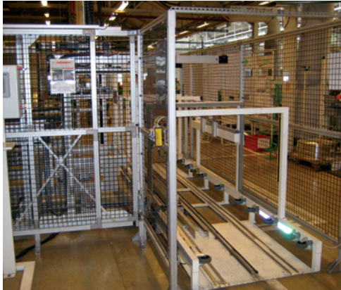
Quick-Guard Standard assembled with mesh.
