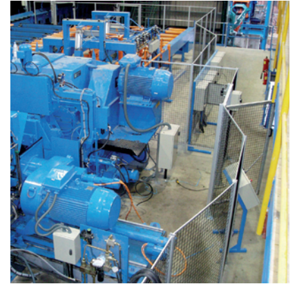
Quick-Guard E with few components and easy to angle at up to 45°.
