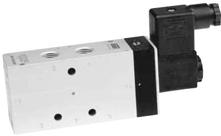
Series KM-10 5/2- and 5/3-way, G 1/4, 2100 NI/min (2.134 Cv)
