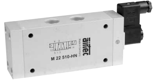
Series M-22 3/2-, 5/2- and 5/3-way, G 1/2, 3300 NI/min (3.354 Cv)
