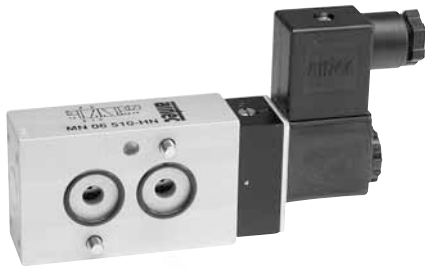
Series MN-06 3/2-, 5/2- and 5/3-way according to NAMUR , 750 NI/min (0.762 Cv)
