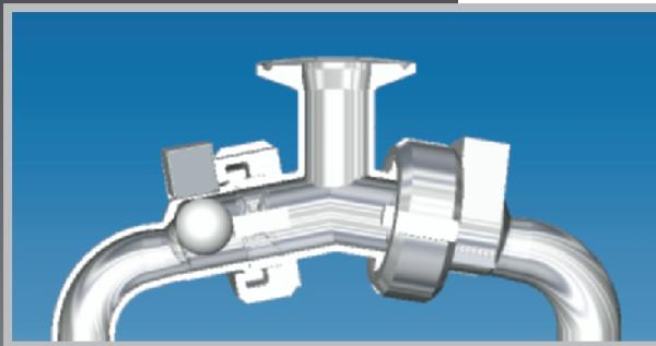
Always a demand for sterile applications: all housing parts of the BIOCOR pumps show no horizontal areas. Each pump comes with four ball lifting magnets, which can be attached to the pump housing from the outside at the location of the four ball valves. The ball valves are risen up magnetically out of their seats and the pump is drained entirely without having to be dismounted. There are no mechanical ball lifters with parts and seals in the wetted area.
