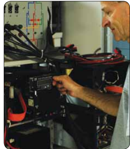
Refurbished equipment is put through a rigorous burn-in cycle to identify marginal components.
