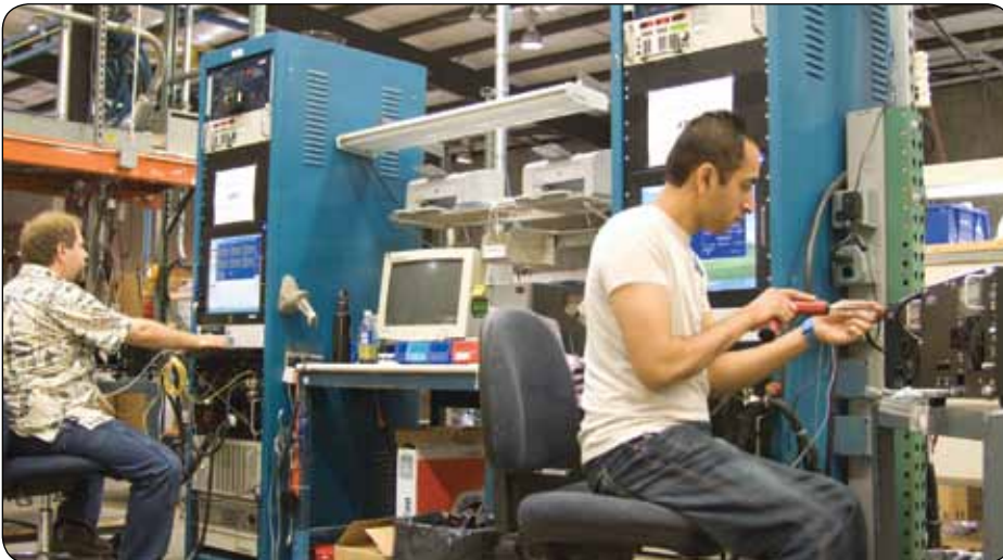
Automated test equipment is used to efficiently verify all functions of refurbished power supplies.
