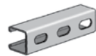
AS 200EH Channel with Elongated Holes Size: 1 5 / 8 " x 1 5 / 8 " x 12 GA. 9 1 / 16 " x 1 1 / 8 " Elongated Holes on 2" Centers. Page 23
