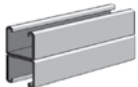
AS 200EH BTB Welded Channel Size: 1 5 / 8 " x 3 1 / 4 " x 12 GA. Two Pcs. AS 200EH Welded Back-to-Back. 9 1 / 16 " x 1 1 / 8 " Elongated Holes on 2" Centers. Page 24
