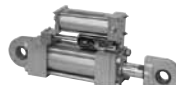
Fig. 200 & C-200 / Fig. 201 & C-201 Hydraulic Shock & Sway Suppressor (Snubber) Size Range: Seven standard sizes with cylinder bores of 1 1/2" to 8" with normal load ratings from 3,000 (LBS) to 128,000 (LBS). All are available with 5", 10", 15" or 20" strokes except the 1 1/2" size which is offered with 5" and 10" strokes only. Snubbers are available with integral or remote reservoirs.
