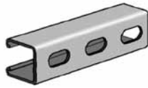
AS 210EH SS/ZTC/HG Channel with Elongated Holes Size: 1 5 / 8 " x 1 5 / 8 " x 14 GA. 9/16" x 1 1 / 8 " Elongated Holes on 2" Centers. Page 77
