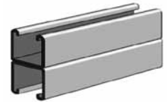
AS 200EH BTB SS/ZTC/HG Welded Channel Size: 1 5 / 8 " x 3 1 / 4 " x 12 GA. Two Pcs. AS 200EH Welded Back-to-Back. 9/16" x 1 1 / 8 " Elongated Holes on 2" Centers Page 75
