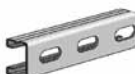
AS 560EH Channel with Elongated Holes Size: 1 5 / 8 " x 1 3 / 16 " x 16 GA. 9/16" x 1 1 / 8 " Elongated Holes on 2" Centers. Page 36
