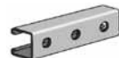
AS 400H Channel with Holes Size: 1 5 / 8 " x 1" x 12 GA. 9/16" Holes on 1 7 / 8 " Centers. Page 30
