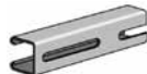
AS 520S Channel with Long Slots Size: 1 5 / 8 " x 1 3 / 16 " x 12 GA. 1 3 / 32 " x 3" Slots on 4" Centers. Page 34
