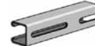
AS 400S Channel with Long Slots Size: 1 5 / 8 " x 1" x 12 GA. 1 3 / 32 " x 3" Slots on 4" Centers. Page 30
