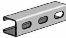
AS 200EH SS/ZTC/HG Channel with Elongated Holes Size: 1 5 / 8 " x 1 5 / 8 " x 12 GA. 9/16" x 1 1 / 8 " Elongated Holes on 2" Centers. Page 75
