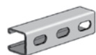
AS 210EH Channel with Elongated Holes Size: 1 5 / 8 " x 1 5 / 8 " x 14 GA. 9 1 / 16 " x 1 1 / 8 " Elongated Holes on 2" Centers. Page 26
