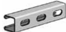
AS 400EH Channel with Elongated Holes Size: 1 5 / 8 " x 1" x 12 GA. 9/16" x 1 1 / 8 " Elongated Holes on 2" Centers. Page 30
