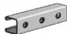
AS 500H Channel with Holes Size: 1 5 / 8 " x 1 3 / 16 " x 14 GA. 9/16" Holes on 1 7 / 8 " Centers. Page 32
