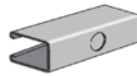
AS 150KO Channel with Knock Outs Size: 1 5 / 8 " x 2 7 / 16 " x 12 GA. 7 1 / 8 " Knock Outs on 6" Centers. Page 21
