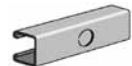
AS 400KO Channel with Knock Outs Size: 1 5 / 8 " x 1" x 12 GA. 7/8" Knock Outs on 6" Centers. Page 30
