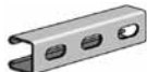
AS 500EH Channel with Elongated Holes Size: 1 5 / 8 " x 1 3 / 16 " x 14 GA. 9/16" x 1 1 / 8 " Elongated Holes on 2" Centers. Page 32
