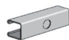
AS 200KO Channel with Knock Outs Size: 1 5 / 8 " x 1 5 / 8 " x 12 GA. 7 1 / 8 " Knock Outs on 6" Centers. Page 23
