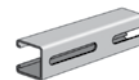
AS 200S Channel with Long Slots Size: 1 5 / 8 " x 1 5 / 8 " x 12 GA. 1 3 / 32 " x 3" Slots on 4" Centers. Page 23
