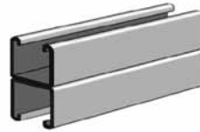
AS 200BTB SS/ZTC/HG Welded Channel Size: 1 5 / 8 " x 3 1 / 4 " x 12 GA. Two Pcs. AS 200 Welded Back-to-Back. Pages 74 & 75
