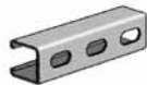
AS 300EH Channel with Elongated Holes Size: 1 5 / 8 " x 1 3 / 8 " x 12 GA. 9/16" x 1 1 / 8 " Elongated Holes on 2" Centers. Page 28
