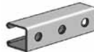
AS 300H Channel with Holes Size: 1 5 / 8 " x 1 3 / 8 " x 12 GA. 9/16" Holes on 1 7 / 8 " Centers. Page 28
