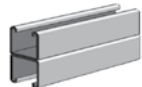
AS 200BTB Welded Channel Size: 1 5 / 8 " x 3 1 / 4 " x 12 GA. Two Pcs. AS 200 Welded Back-to-Back. Pages 22 & 24
