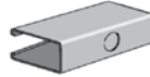
AS 100KO Channel with Knock Outs Size: 1 5 / 8 " x 3 1 / 4 " x 12 GA. 7 1 / 8 " Knock Outs on 6" Centers. Page 19
