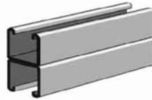
AS 210BTB SS/ZTC/HG Welded Channel Size: 1 5 / 8 " x 3 1 / 4 " x 14 GA. Two Pcs. AS 200 Welded Back-to-Back. Pages 76 & 77
