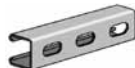
AS 520EH Channel with Elongated Holes Size: 1 5 / 8 " x 1 3 / 16 " x 12 GA. 9/16" x 1 1 / 8 " Elongated Holes on 2" Centers. Page 34
