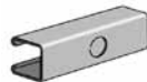
AS 300KO Channel with Knock Outs Size: 1 5 / 8 " x 1 3 / 8 " x 12 GA. 7/8" Knock Outs on 6" Centers. Page 28
