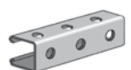
AS 200H3 Channel with Holes on all Three Sides Size: 1 5 / 8 " x 1 5 / 8 " x 12 GA. 9 1 / 16 " Holes on all three sides are on 1 7 / 8 " Centers. Page 23
