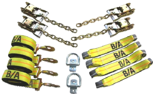
Part # 38-200D Roll Back Tie-Down System Consists of: 38-200-L (4) 14' Long straps with snap hook 38-200-S (4) Short straps with sewn eyes 38-100-R (4) Ratchets with chain 38-DR1 (2) Bolt on Forged D-Rings
