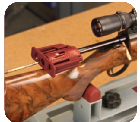
4. Insert cleaning rod with jag, penetrating patch and releasing it
