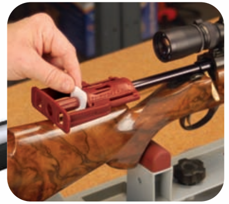
1. With the sliding rear guide pulled out, center the patch with access hole
