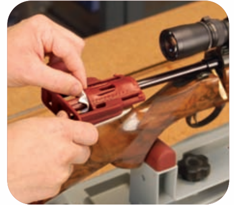
2. Push the sliding rear guide forward, securing the patch
