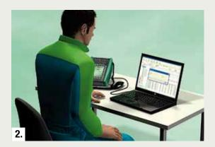
Download calibration procedures and instructions from the Beamex® CMX Calibration Software to Beamex® Multifunction Calibrators.
