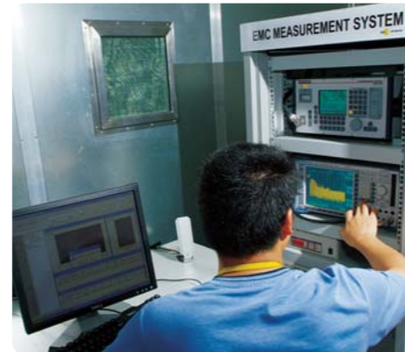
This is the Electromagnetic chamber where we test all products for compliance with standards such as FCC emissions, CE and safety. The facility represents a multi-million dollar investment and includes at least one machine that goes "ping"
