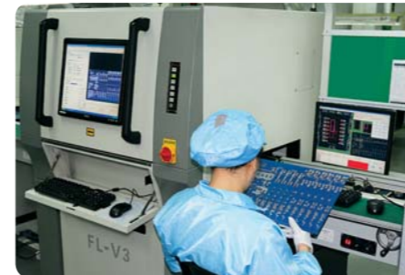
State-of-the-art Auto Optical Inspection System that zooms in on every solder joint
