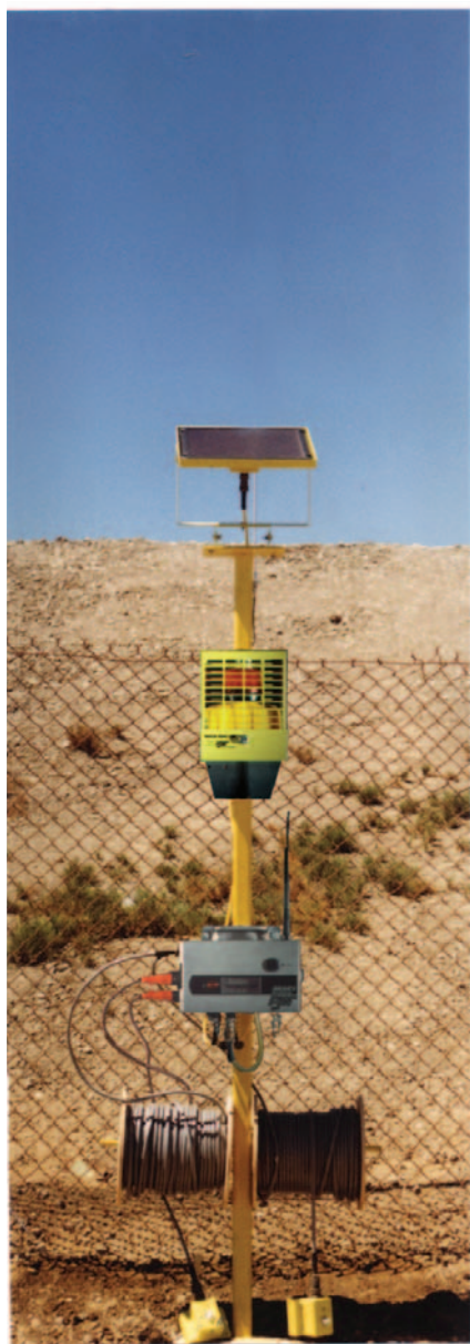
Hazardous Gas Measurement: Monitor Combustibles, Oxygen and/or Toxic gases. Change the gas monitored at any time. Sensors may be remotely placed up to 250 ft (75 meters) away from the Detector.
