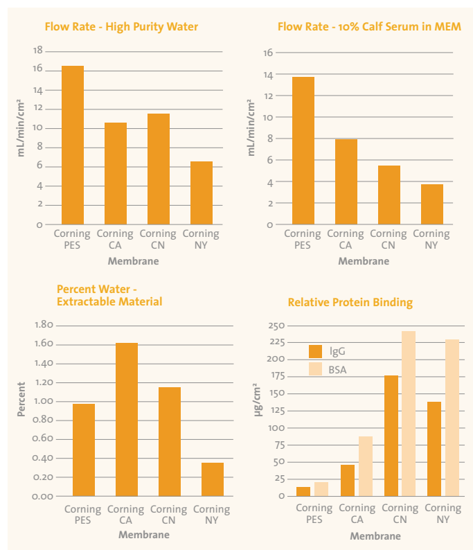
Figure 1. Important Performance Characteristics of Corning® Filter Membranes
