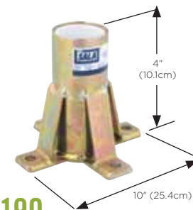
8516190 FLOOR MOUNT SLEEVE Zinc plated mild steel construction. Mounts to horizontal concrete or steel structure. Comes with PVC sleeve liner.
