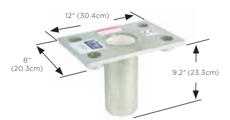
8510316 FLOOR MOUNT SLEEVE Mild steel construction. Recessed fastener pockets allow for bolt-in installation into existing concrete or steel structure. Flush mount design allows passage of traffic and eliminates trip hazards when not in use. Comes with PVC sleeve liner.
