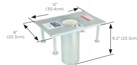
8510311 FLUSH FLOOR MOUNT SLEEVE Mild steel construction. Comes with pins for fresh concrete and cast-in-place concrete anchors for new construction or renovation. Flush mount design allows passage of traffic and eliminates trip hazards when not in use. Comes with PVC sleeve liner.
