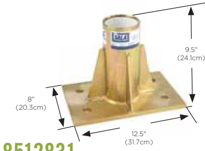
8512831 CENTER MOUNT SLEEVE Zinc plated mild steel construction. Mounts to existing steel and concrete structures by welding or bolting. Comes with PVC sleeve liner.
