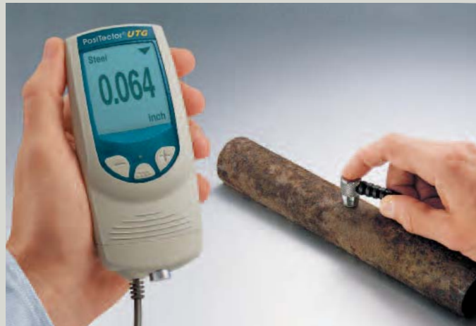
UTG Std measures the remaining wall thickness of steel, and more due to the effects of corrosion and erosion.
