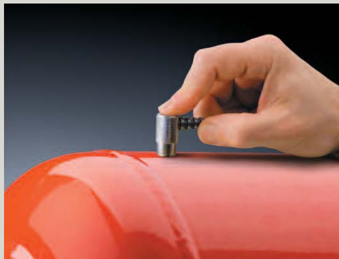
UTG ME Thru-Paint model measures the metal thickness of a painted structure without having to remove the coating.
