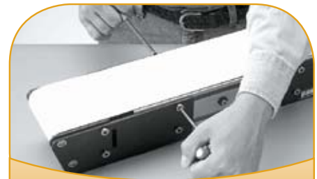
Rack and Pinion Belt Tensioning
