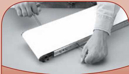
Rack and Pinion Belt Tension
