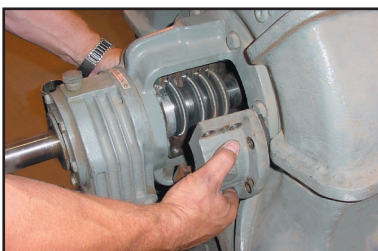
Sealing Gland Housing on the RLA & RLVA is split for easy removal and inspection of carbon rings.
