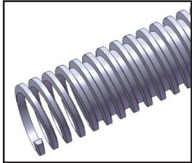
Single Start Screw - Lead & Pitch are the same
