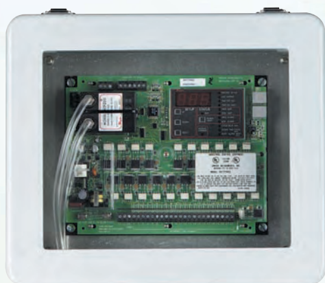
DCT1000 - NEMA 4/4X Weatherproof Enclosure
