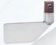
PDL-4. 316 SS single vane paddle for heavy weight materials with a minimum bulk density of 70 lb/ft³ (1122 kg/m³). Fits through 1-1/4" coupling eliminating the need for a mounting flange.
